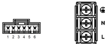
Figure 3 - LPM616 Front Panel Connectors Pinout View
